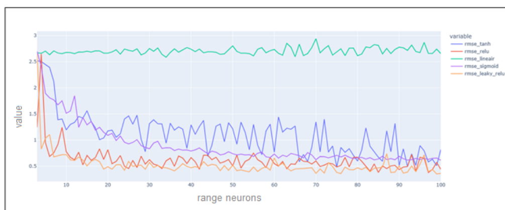
Figure 10. RMSE variations for different numbers of neurons and activations functions
