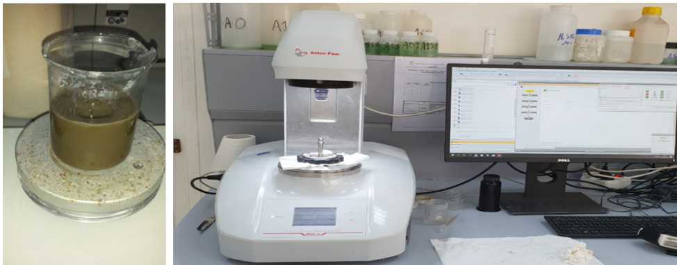
Figure 2. Experimental setup for rheological measurements
