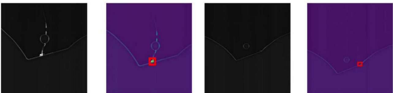
Figure 11. Glass's edge defects
