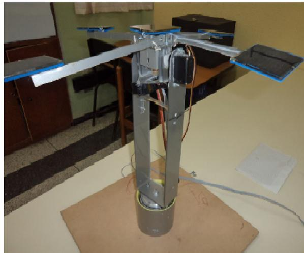
Figure 6. Structure with the inclination of the solar panels
