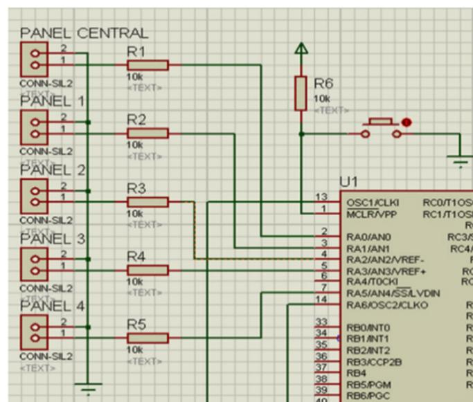
Figure 7. Proteus schematic of voltage sensing circuitry
