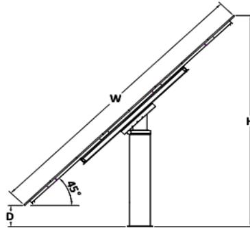
Figure 4. Single-axis solar tracker
