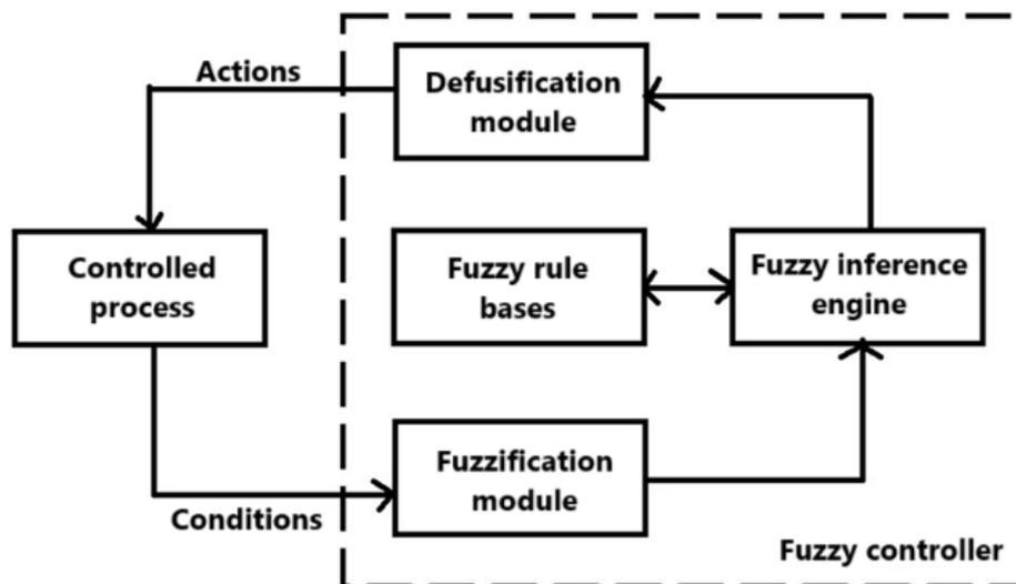
Figure 8. Schematic diagram of a controller based on fuzzy logic<sup>(28)</sup>
