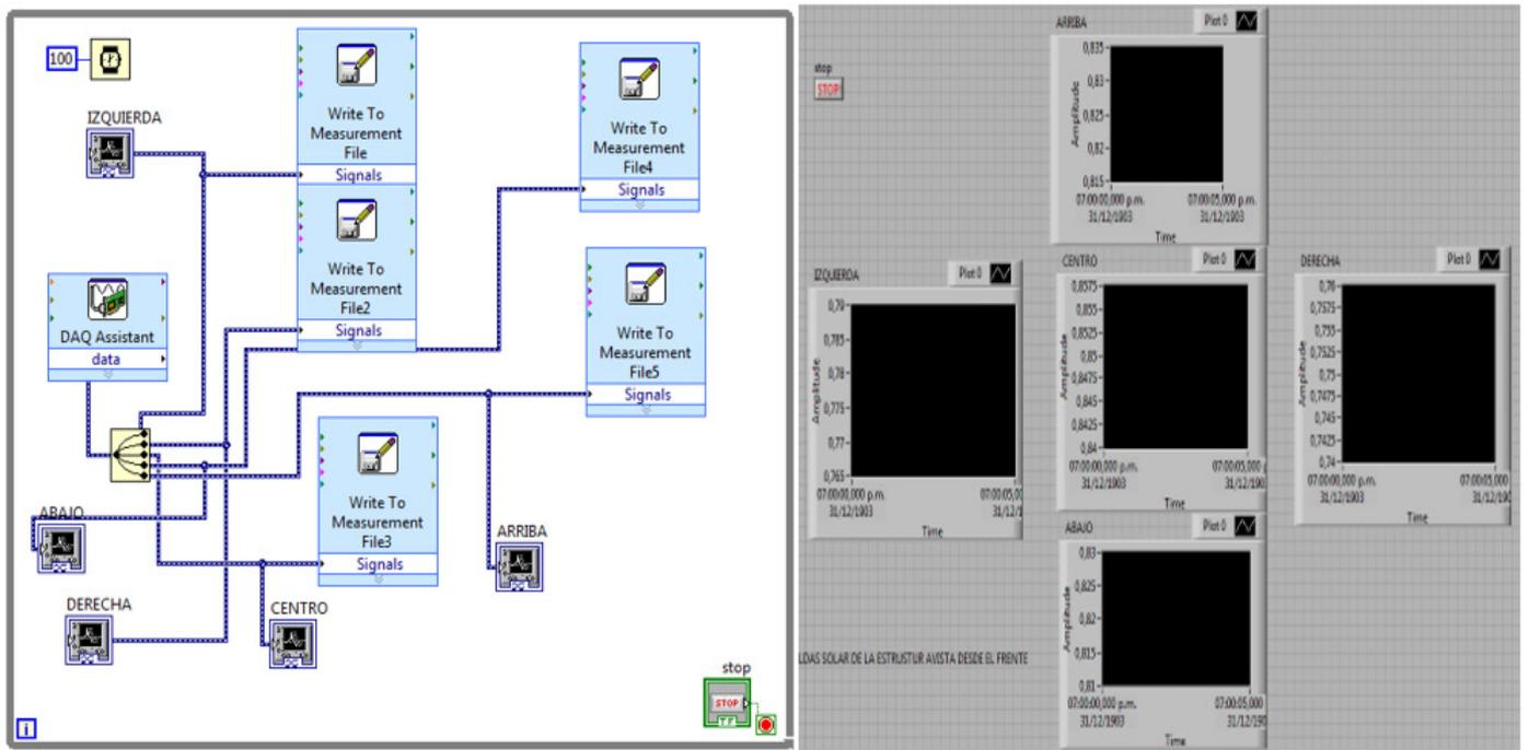
Figure 13. LabVIEW program of the ADQ system
