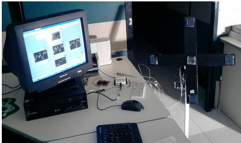
Figure 12. Acquisition software for calibration of Photovoltaic cells
