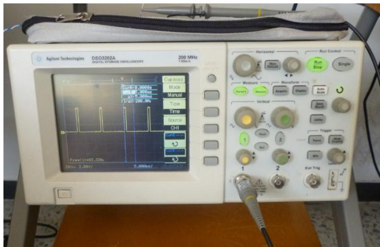
Figure 14. PWM signal at the start position
