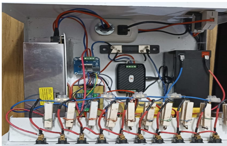
Figure 11. Internal distribution of the components in the emulator prototype
