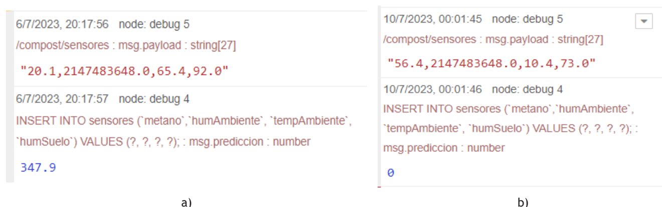
Figure 14. comparative methane levels at NodRed
