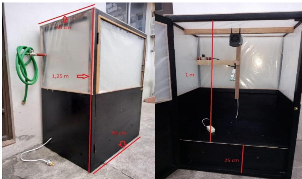
Figure 2. Compost box dimensions
