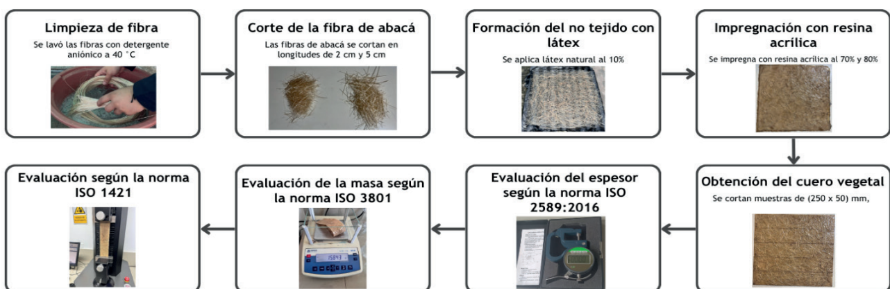
Figure 1. Biocomposite manufacturing process
